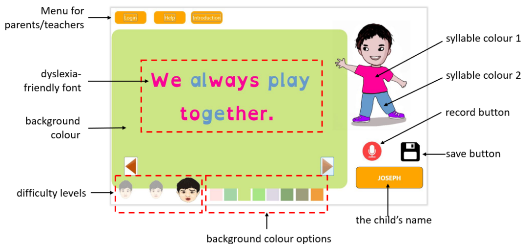
Figure 3. The graphical user interface of BacaDisleksia 2.0, designed to suit dyslexic children's needs, requirements, and preferences.
